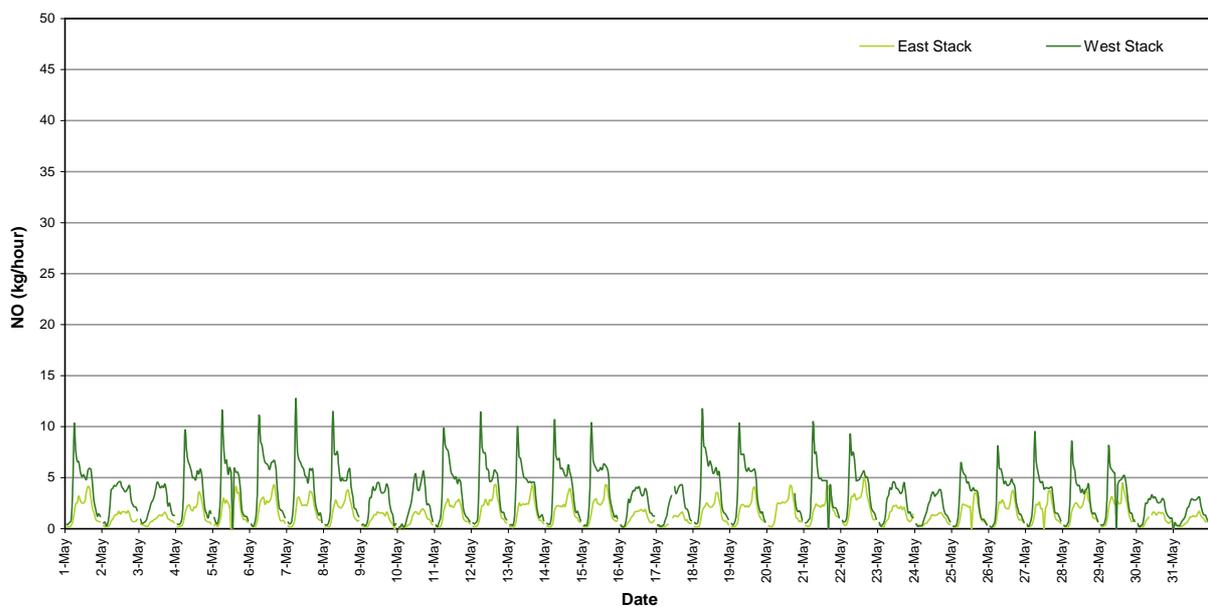
*Figure 11: Nitric Oxide Mass Rate (1 Hour Average)*
