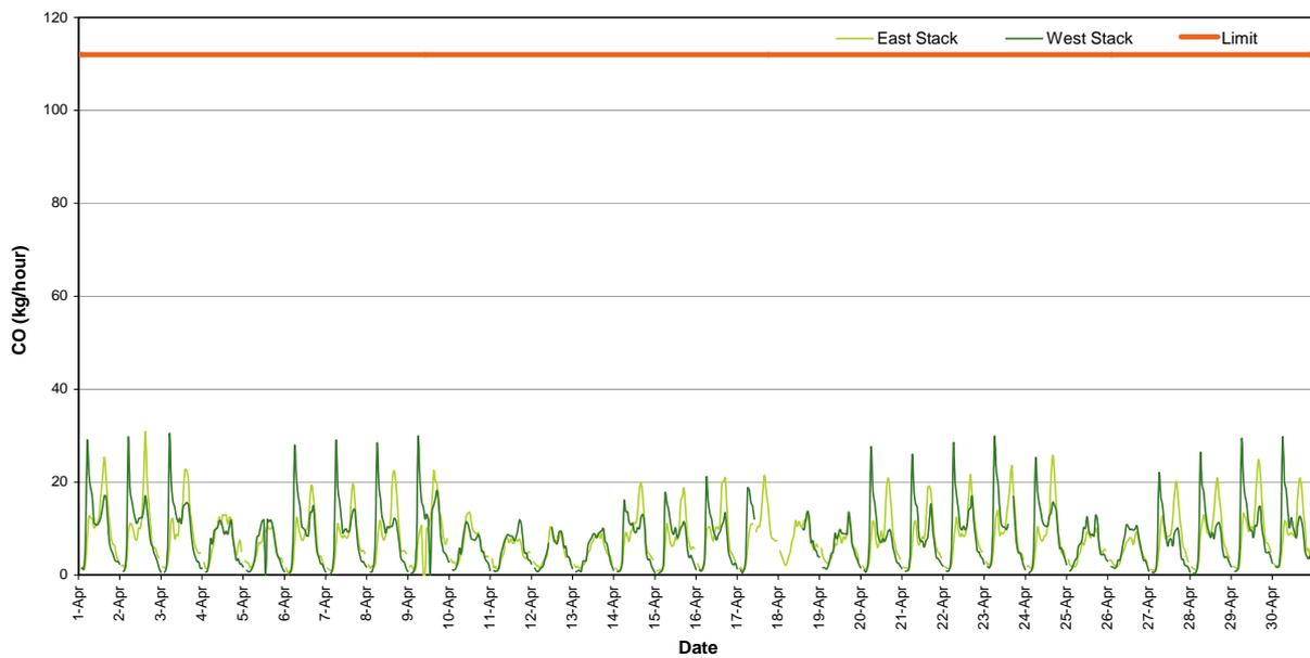
*Figure 4: Carbon Monoxide Mass Rate (1 Hour Average)*
