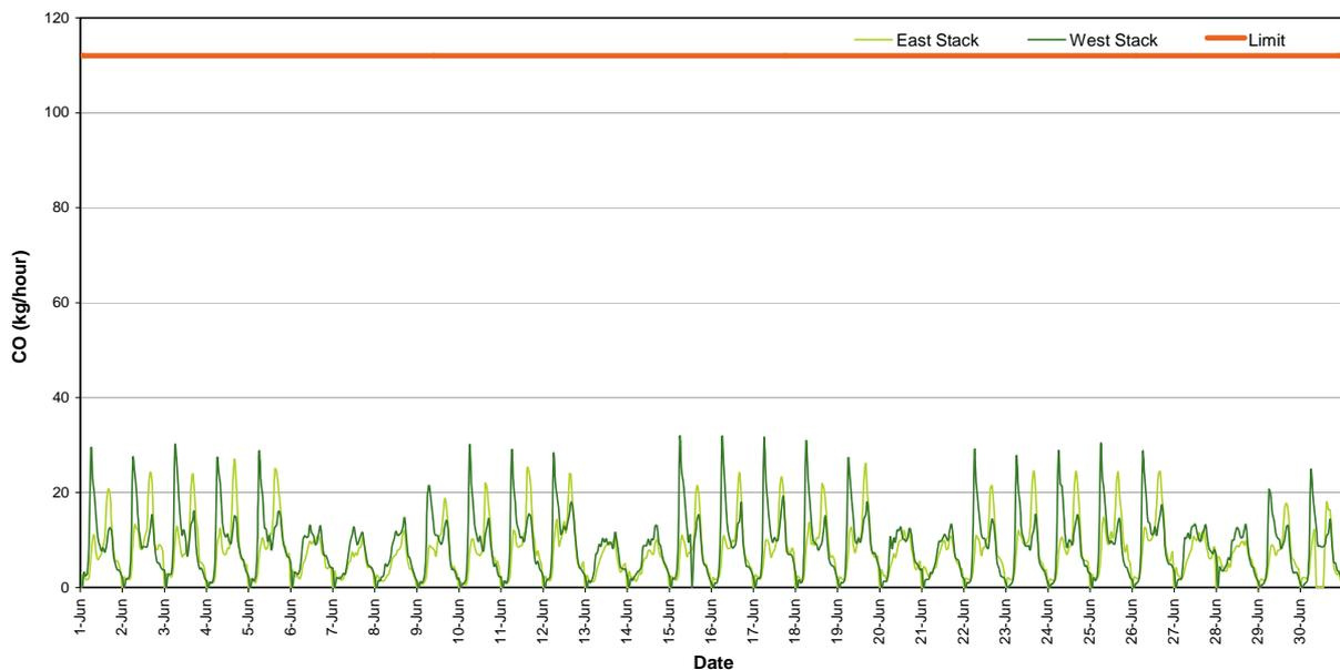
*Figure 16: Carbon Monoxide Mass Rate (1 Hour Average)*
