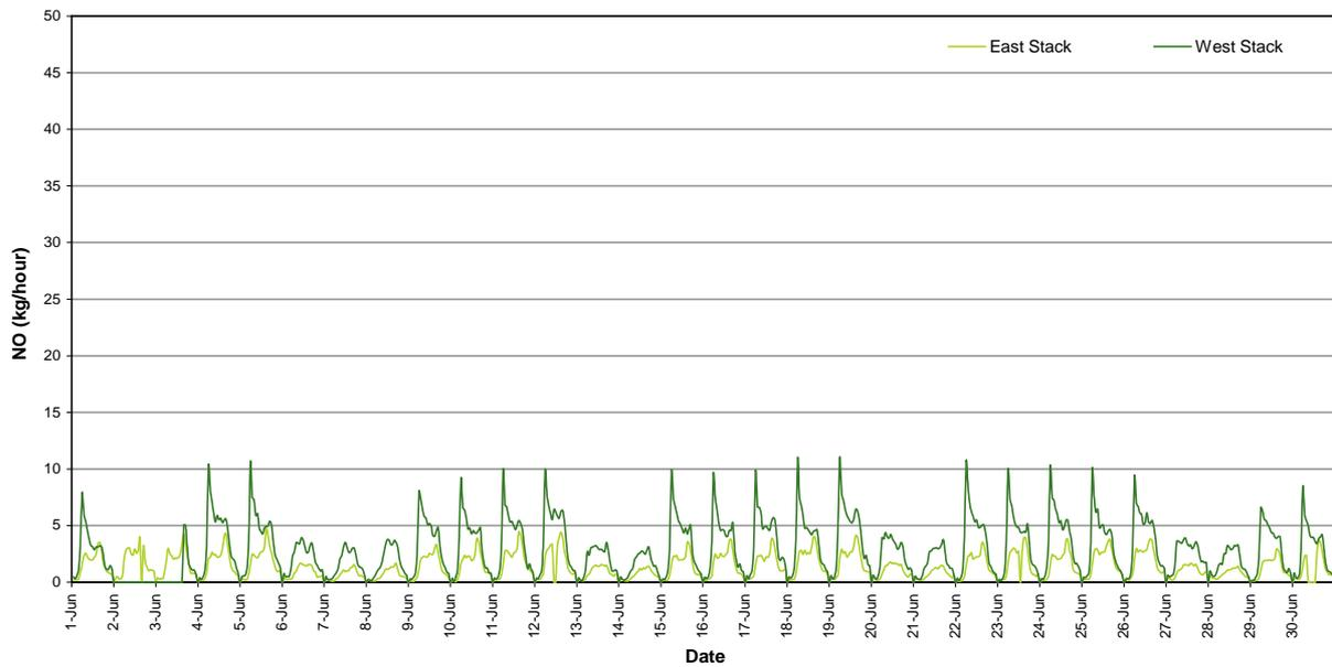
*Figure 17: Nitric Oxide Mass Rate (1 Hour Average)*
