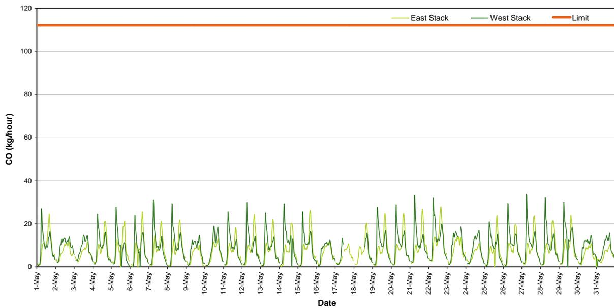
*Figure 10: Carbon Monoxide Mass Rate (1 Hour Average)*
