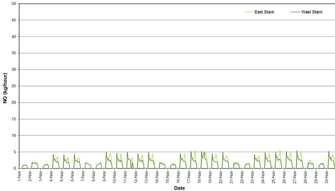
Figure 11: Nitric Oxide Mass Rate (1 Hour Average)
