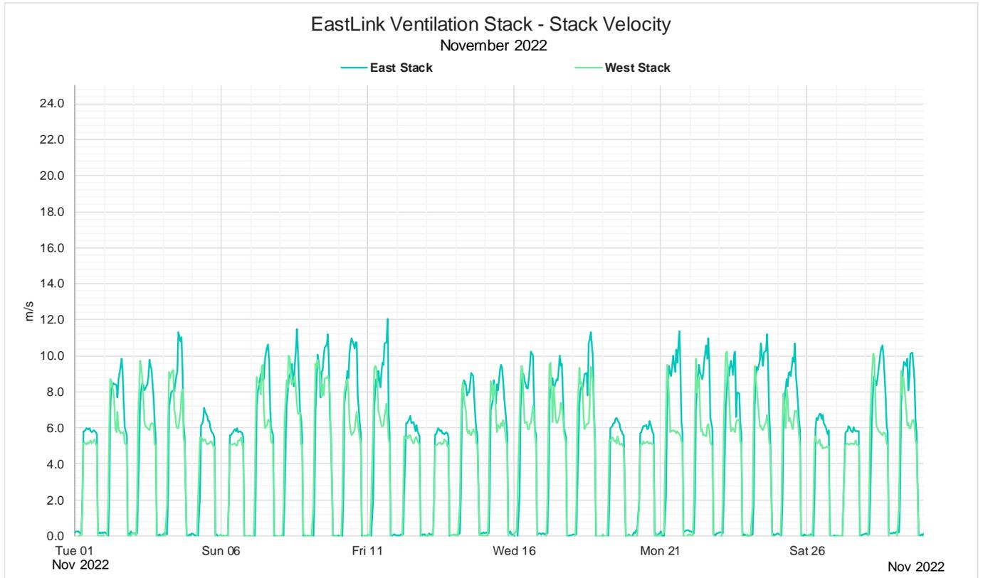
Figure 13: November 2022 Monthly 1 hour average stack velocity
