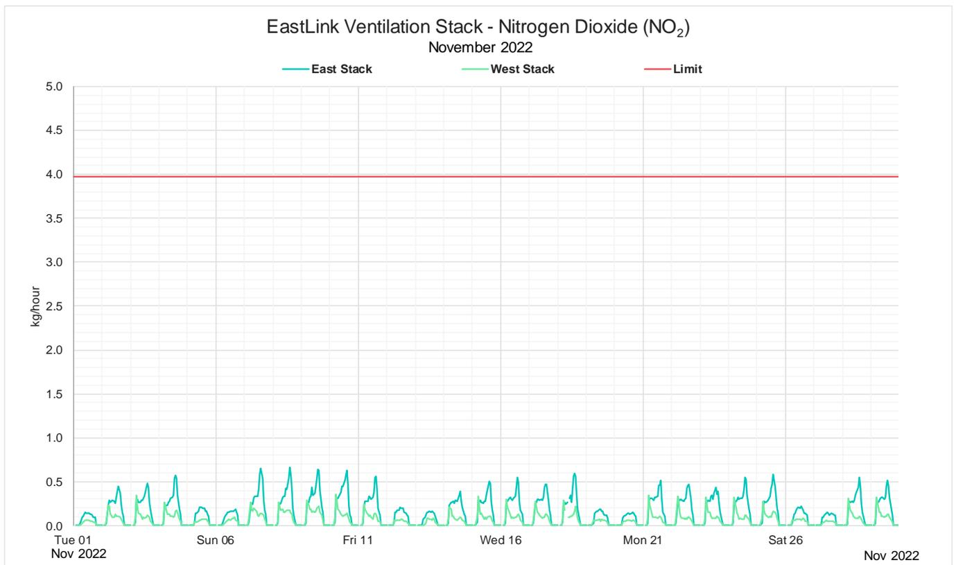
Figure 8: November 2022 Monthly 1 hour mass rate NO<sub>2</sub>
