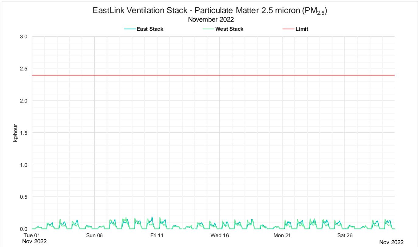
Figure 11: November 2022 Monthly 1 hour mass rate PM<sub>2.5</sub>
