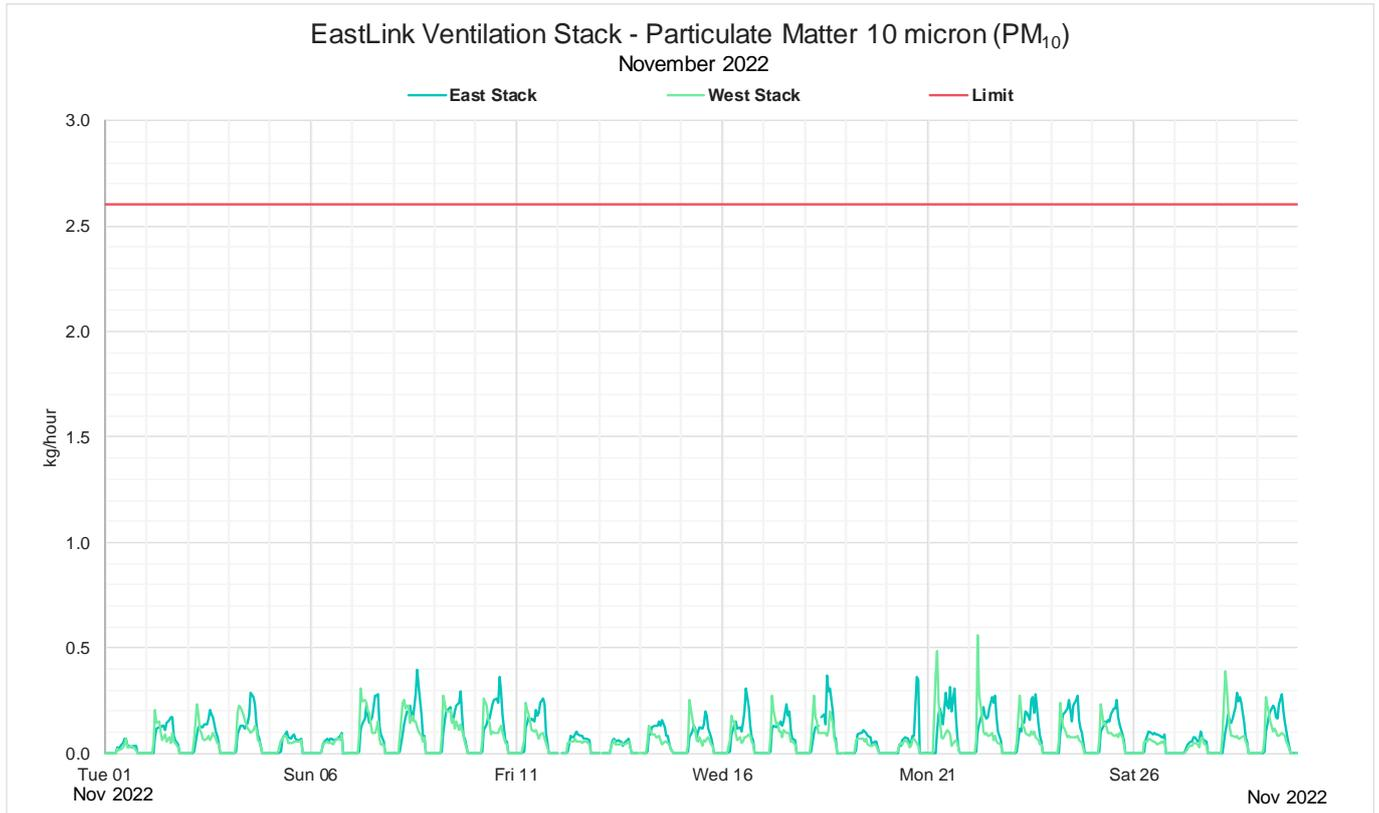
Figure 12: November 2022 Monthly 1 hour mass rate PM<sub>10</sub>
